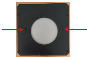
Figure 3: Beam Dump Locking Screws on the Bottom of the Unit
